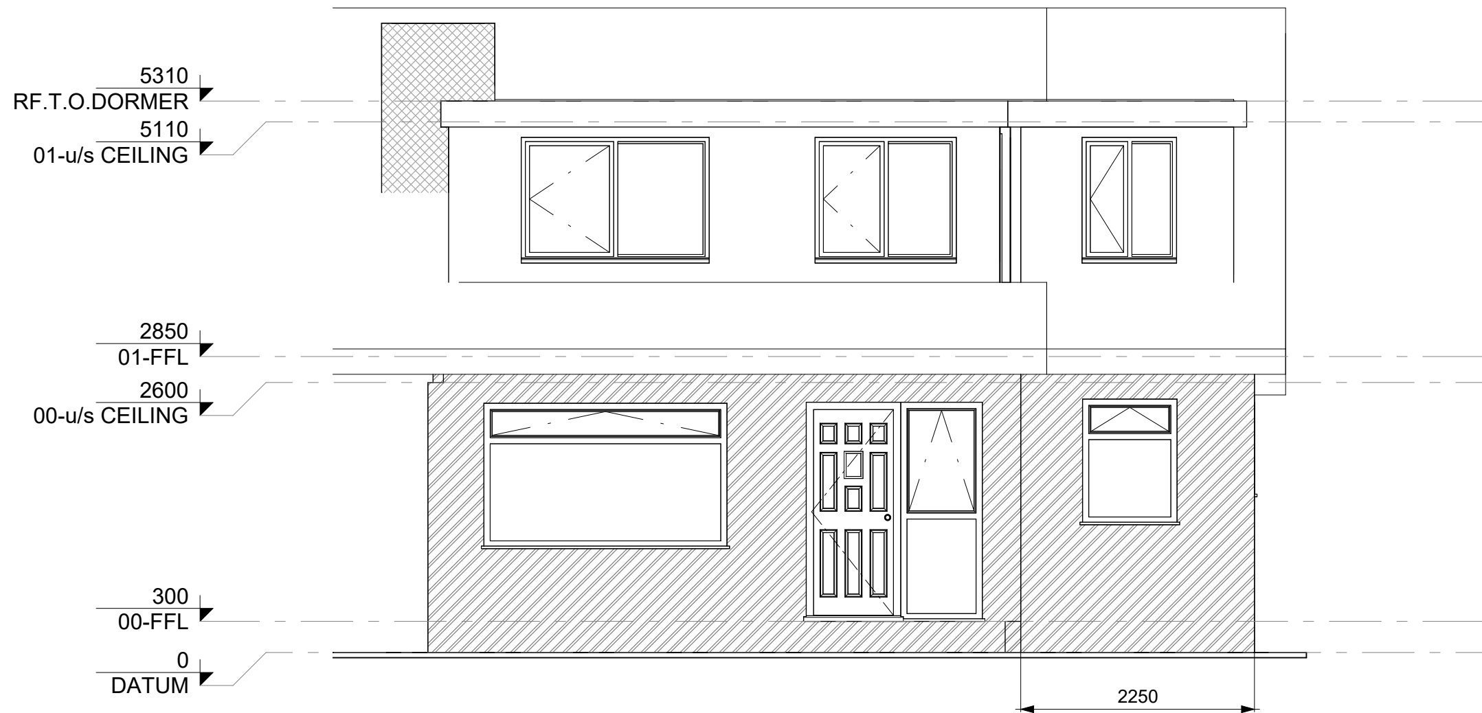
1 PROPOSED FRONT ELEVATION 1 : 50
