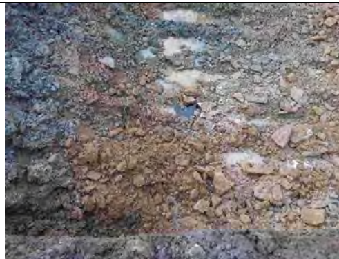
Thin free product (black) on top of groundwater ingress in centre of cell
