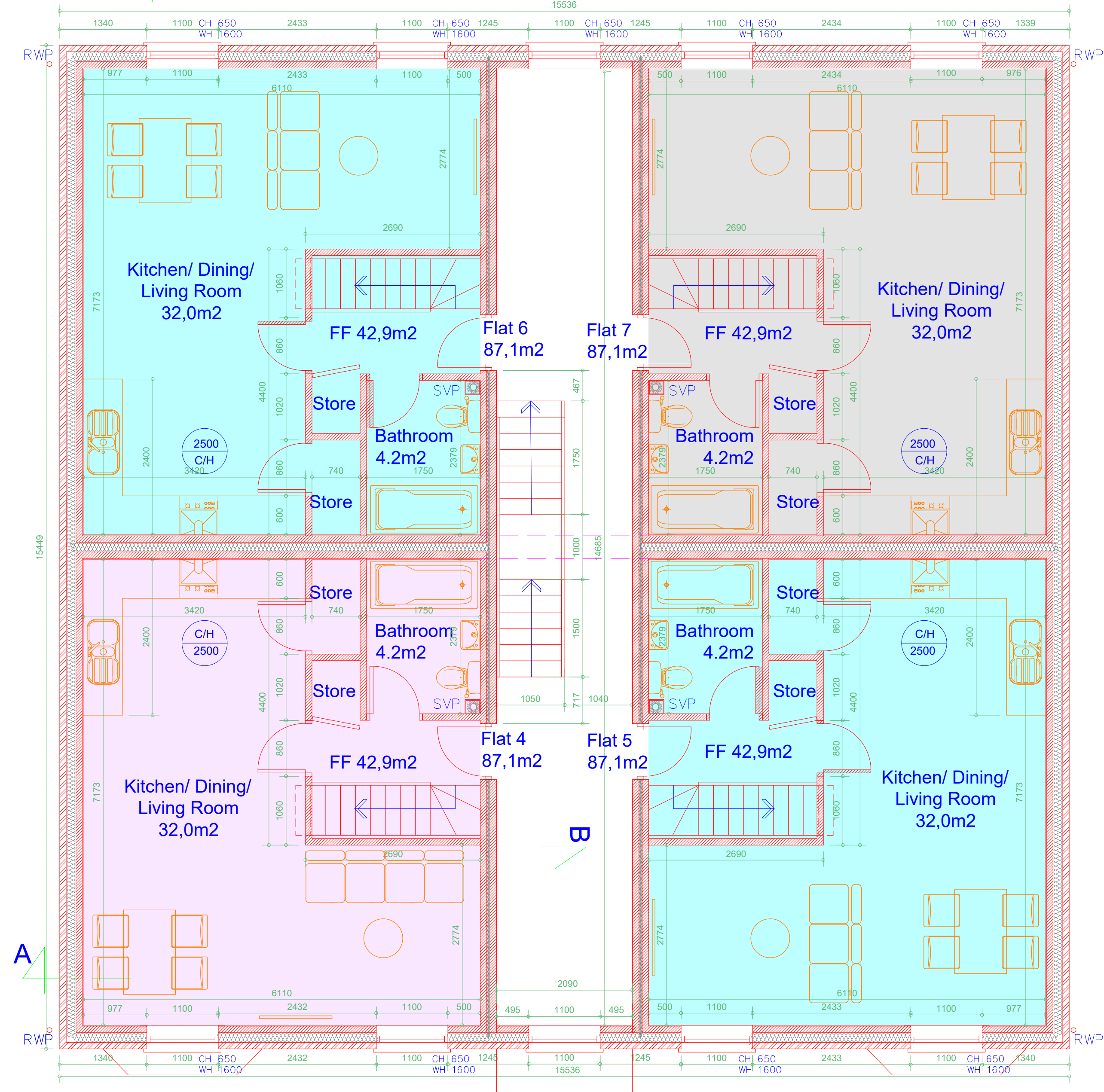
First Floor Plan Scale 1:50
