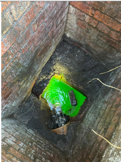
Other Site Photos: MH02 DS MH03 - DYE TEST PROVEN FOR CONNECTIVITY
