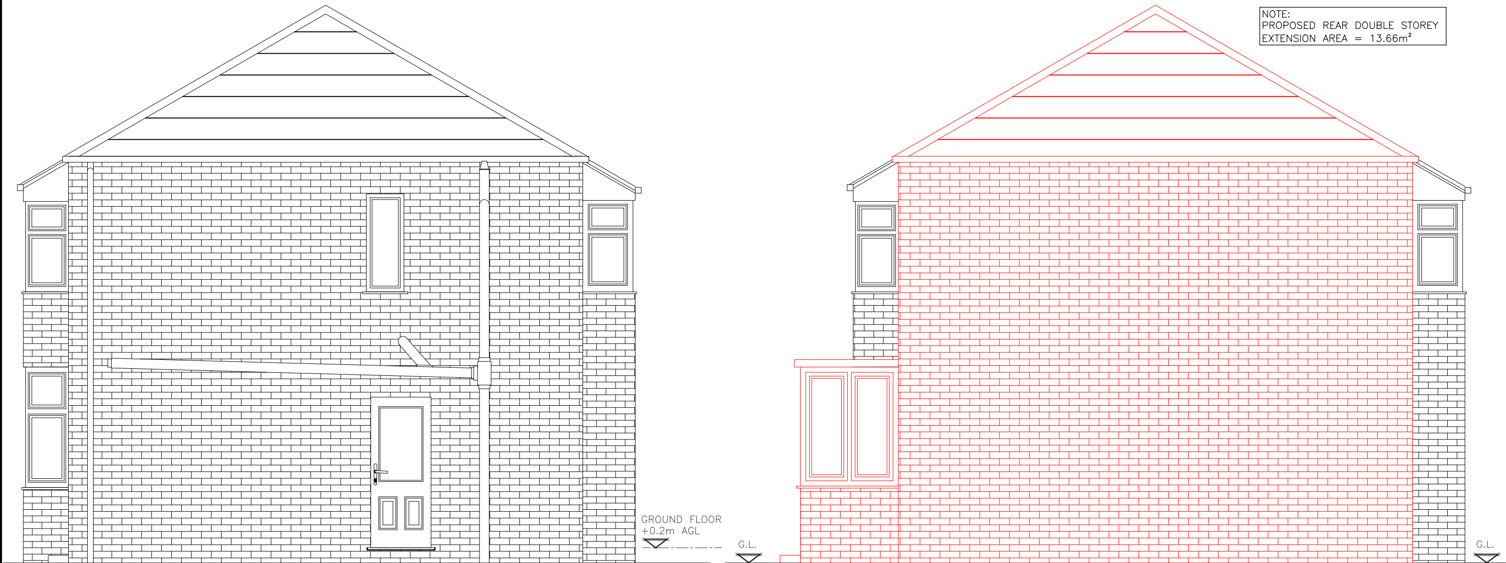
EXISTING SIDE ELEVATION
