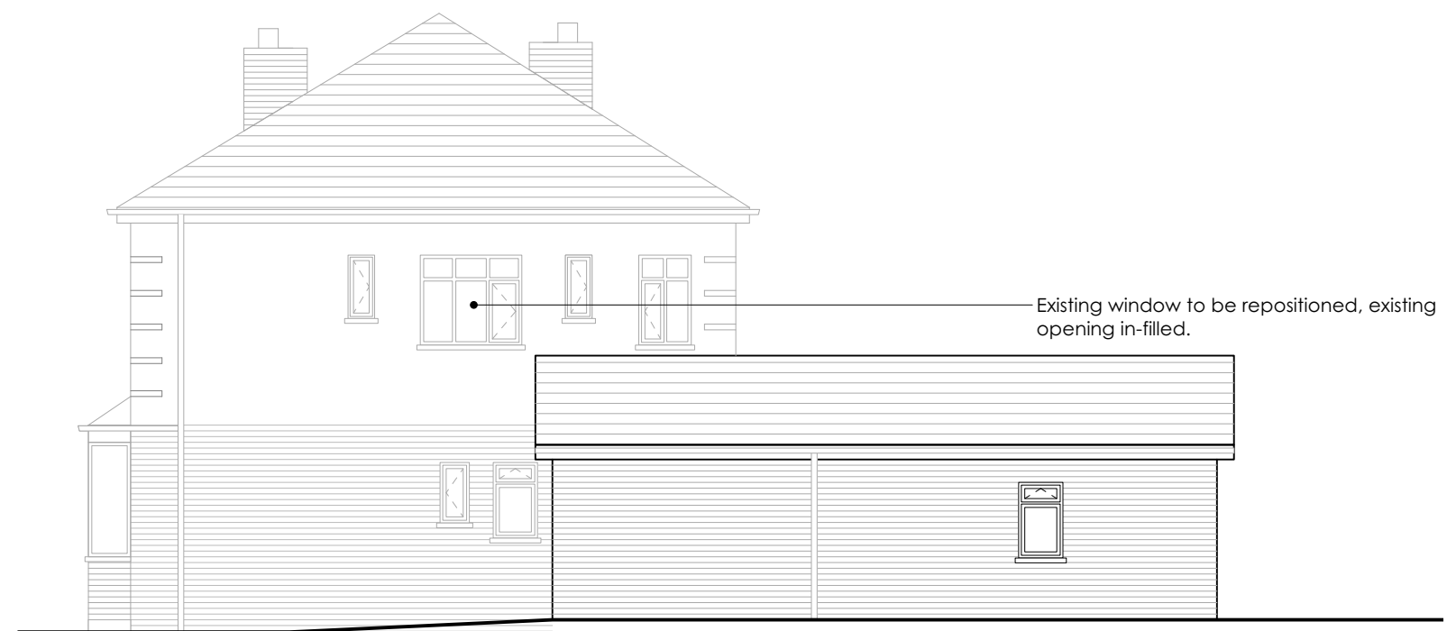
Existing side elevation 1:100
