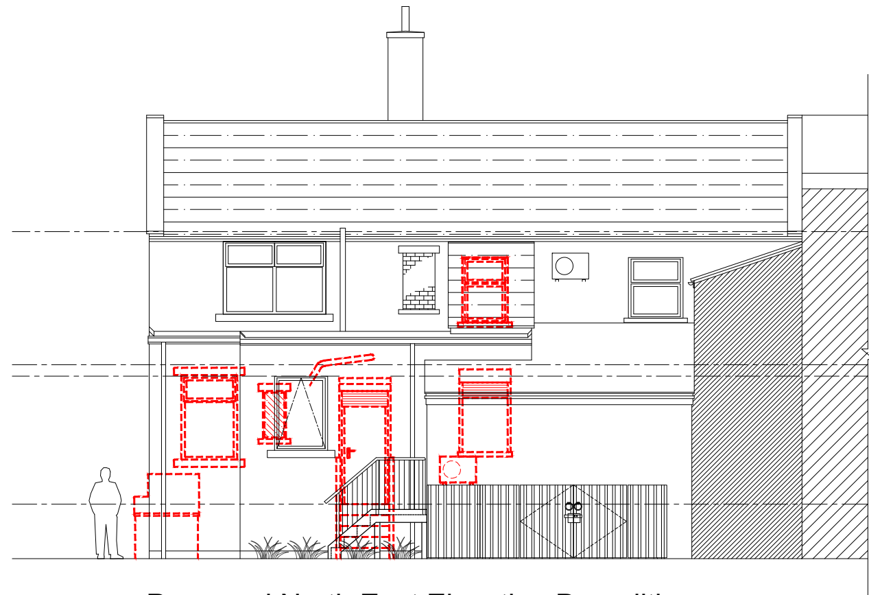
Proposed North East Elevation Demolitions Scale 1:100
