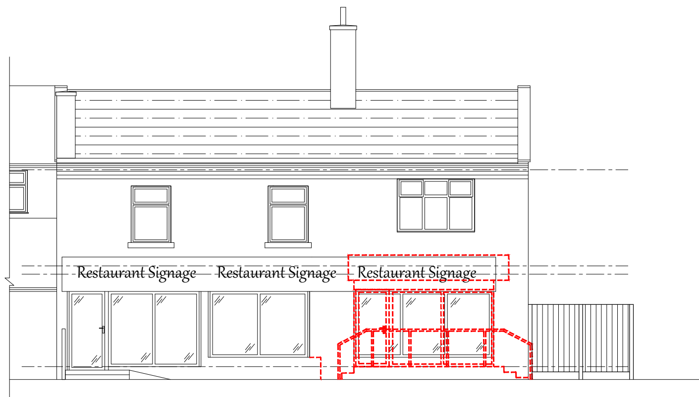
Proposed South West Elevation Demolitions Scale 1:100
