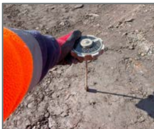
Hand shear vane testing
