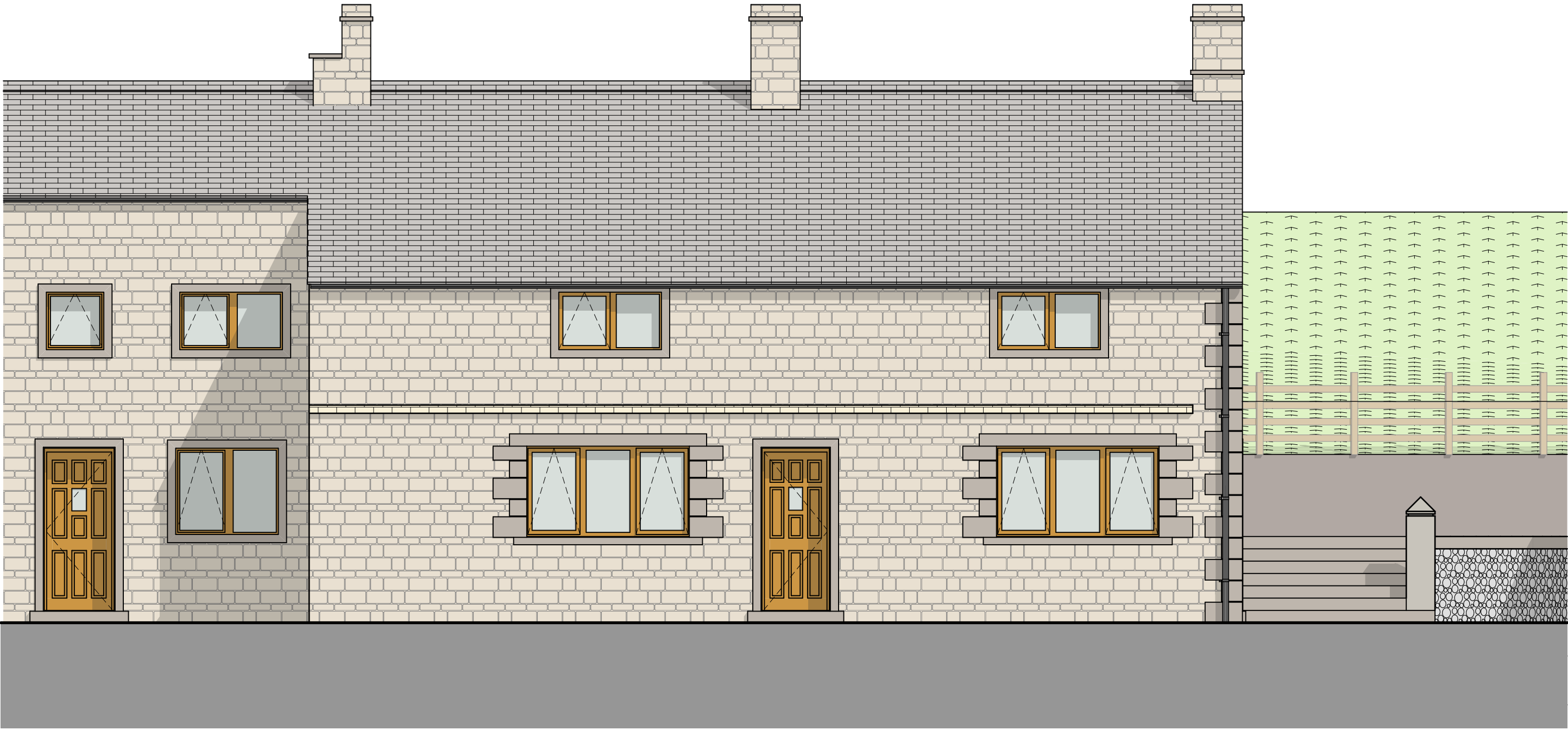
existing south (front) elevation 1:50 @ A1
