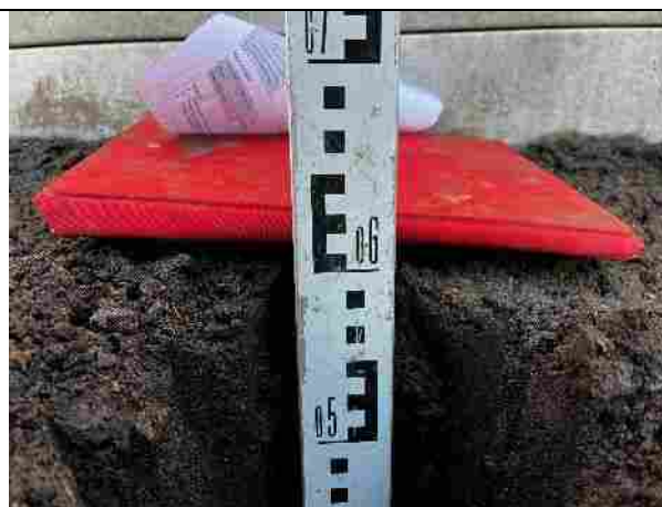
Depth measurement in northeastern landscaped area (circa 600mm soil cover).
