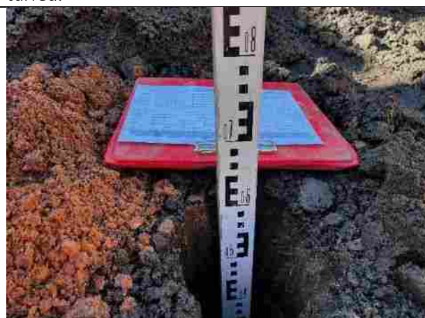
Depth measurement in the rear of Plot 7 (circa 650mm soil cover).
