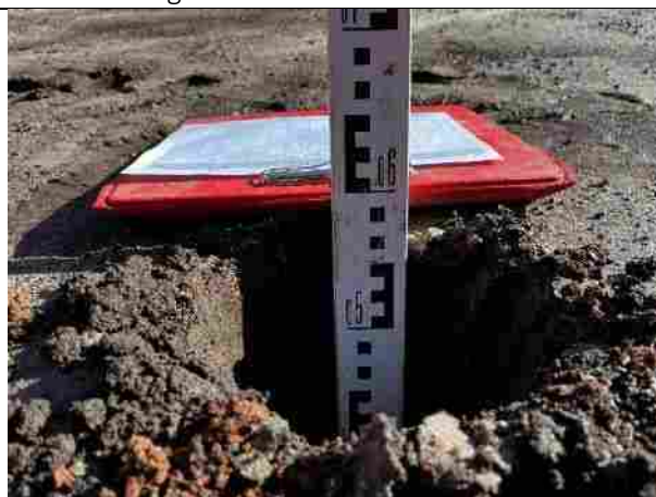
Depth measurement in the rear of Plot 8 (circa 600mm soil cover).
