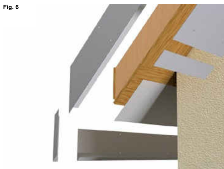
Angled soffit box end construction
