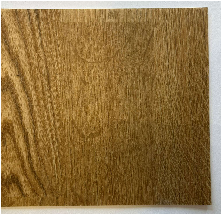
Figure 3- Vinyl flooring to WCs
