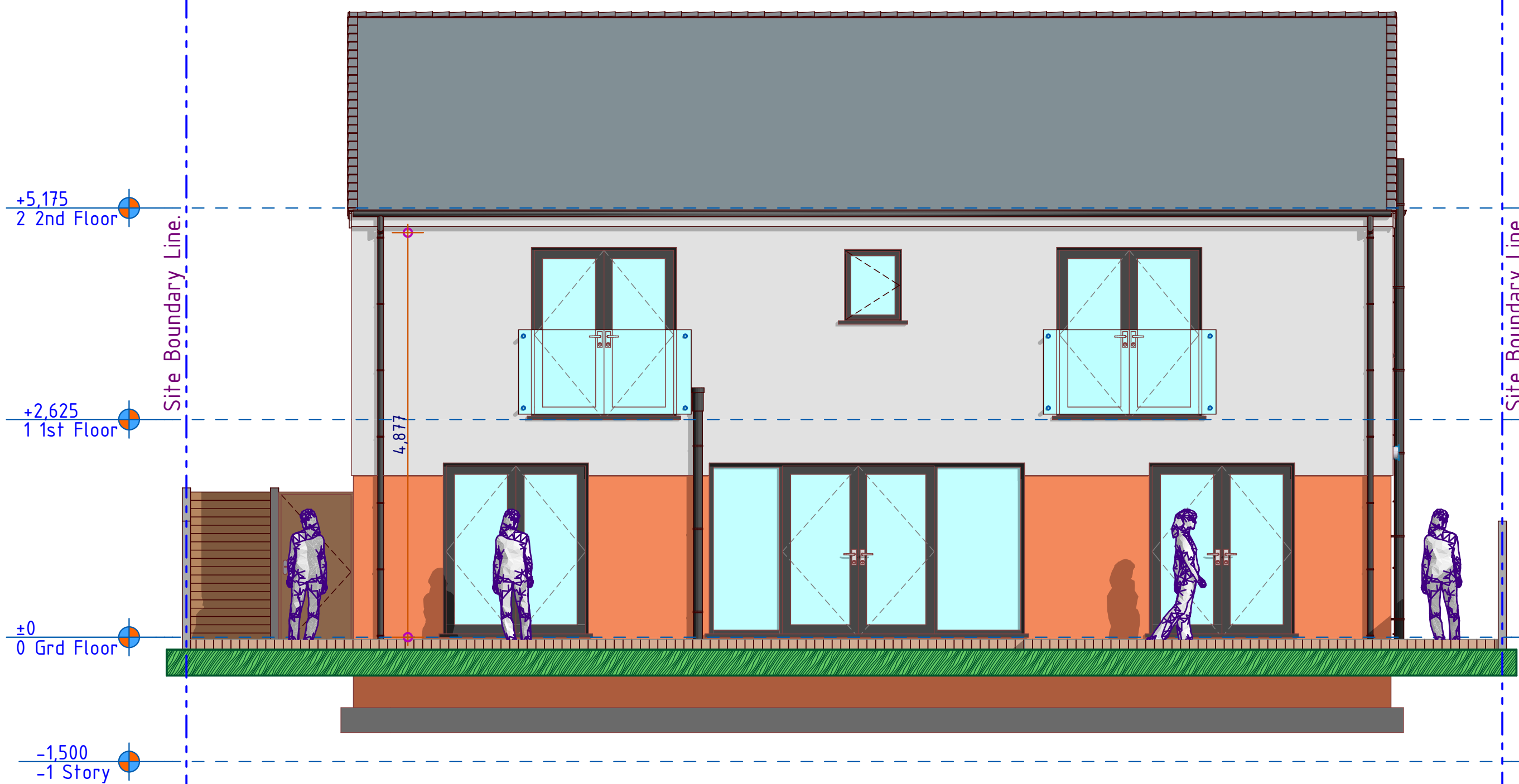
3 Existing Rear Elevation 1:50
