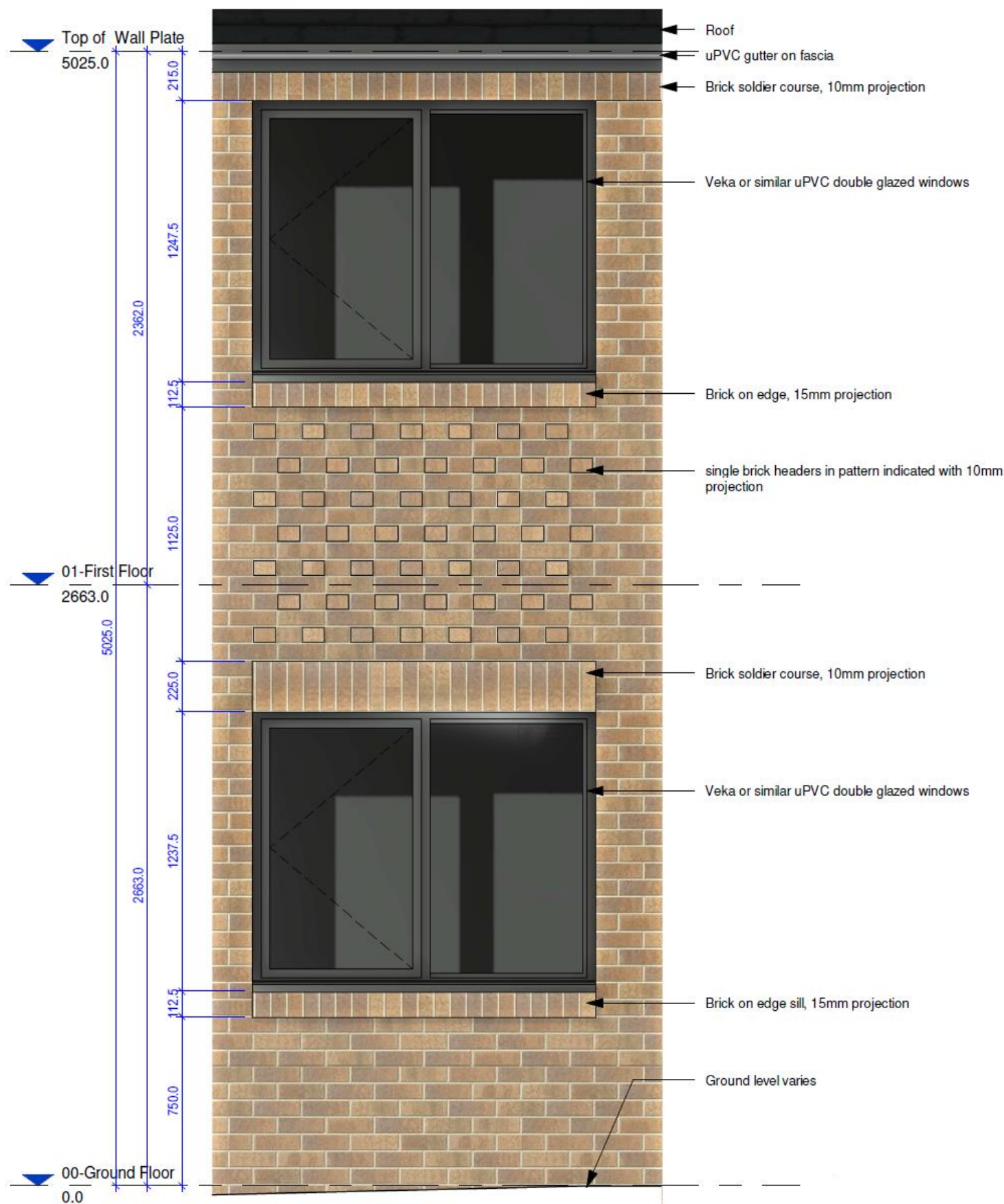
Figure 16 House Brick Detailing Example
