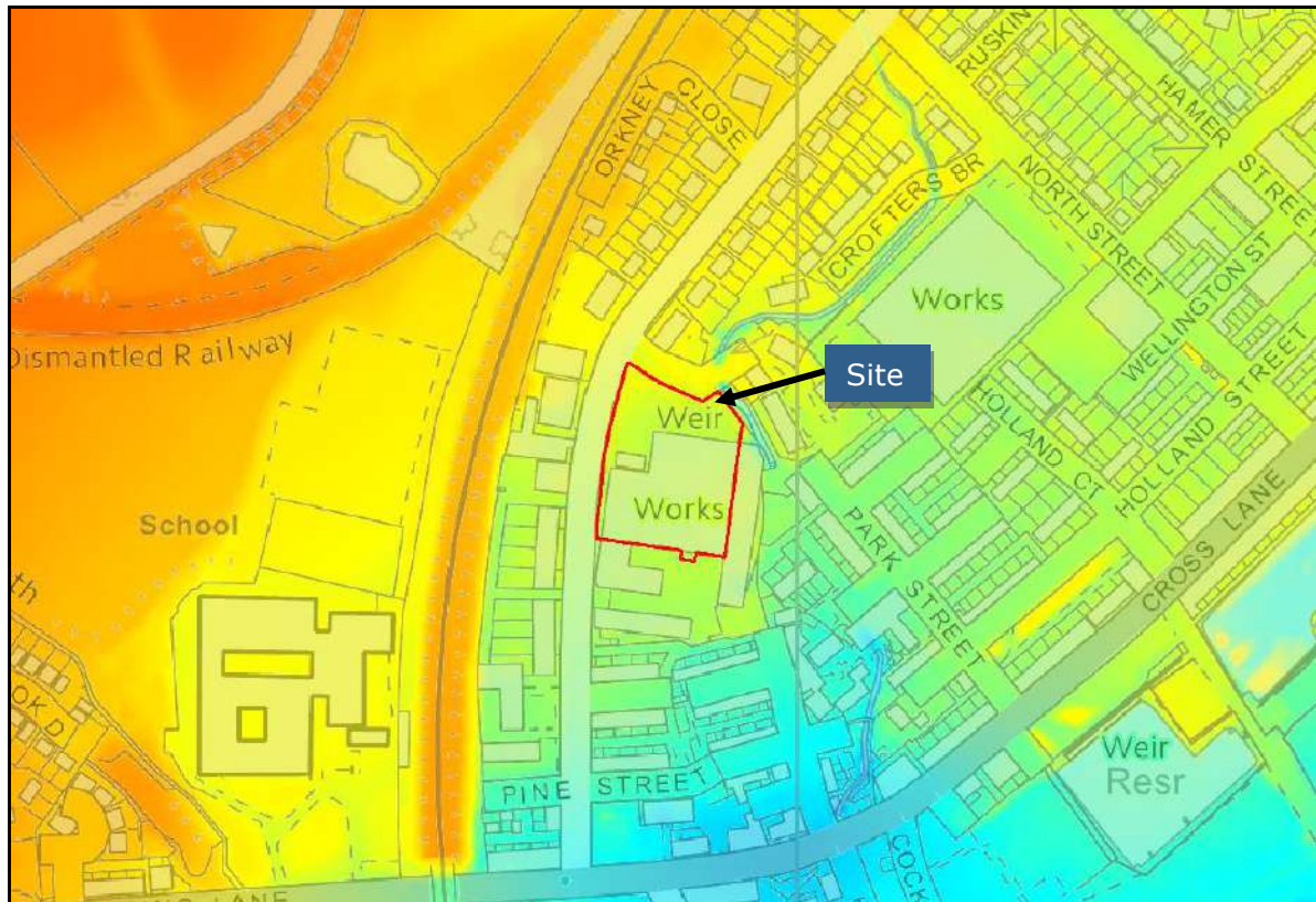
Figure 2: Filtered LIDAR survey data at 1m resolution where higher ground is denoted by red and orange colours and lower ground is denoted by blue colours
