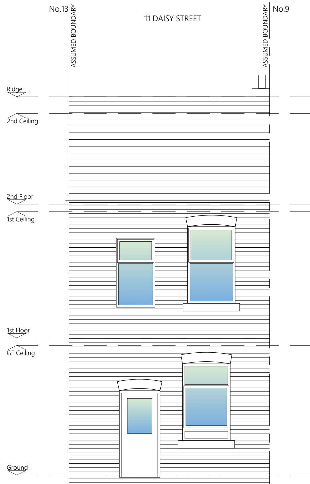
EXISTING REAR ELEVATION
