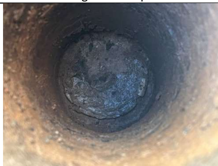
Downhole view of soil in capping layer excavation in rear garden area showing membrane.
