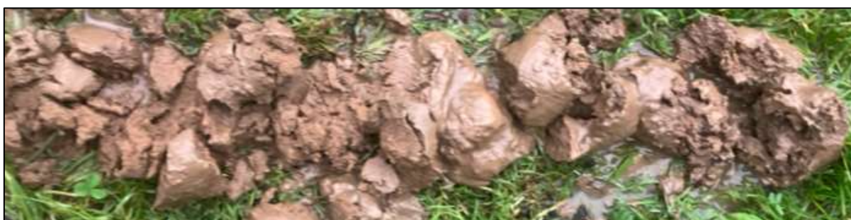
Figure 5-D: Suspected Glacial Till encountered in WLS06.
