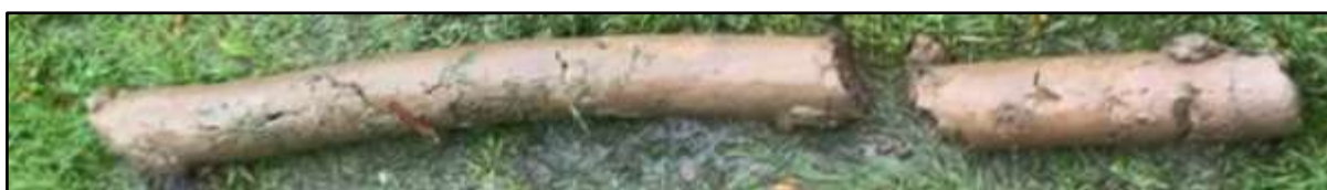
Figure 5-C: Made Ground – Reworked Glacial Till encountered within WLS06 between a depth of 1-2m bgl.
