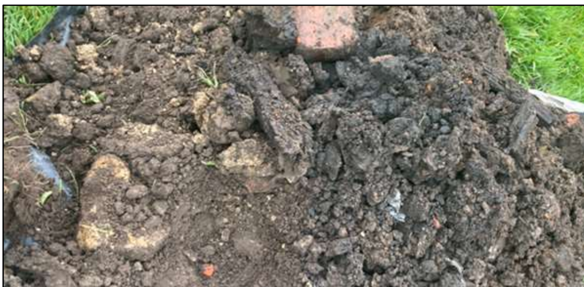
Figure 5-B: Made Ground encountered in HP01
