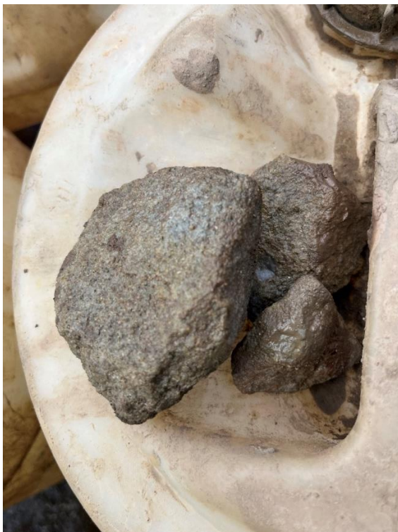
Station Works: 23/07/23 BH02 Granit Boulder 12.50m
