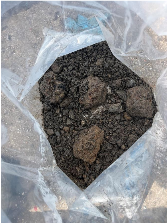
Station Works: 25/07/23 BH03 Made Ground
