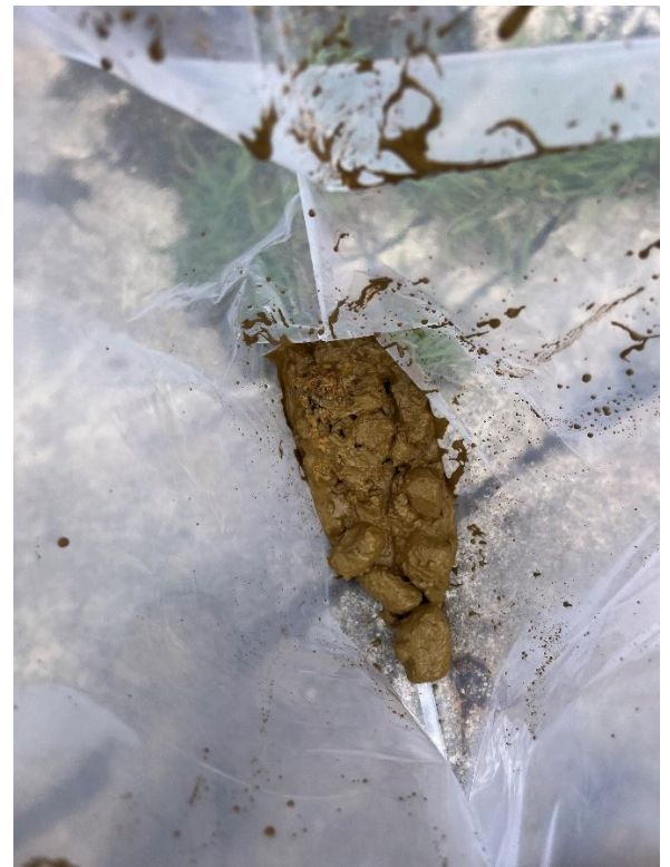
Station Works: 25/07/23 BH04 Sand/Gravel 2.0m
