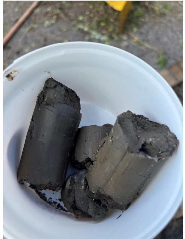
Station Works: 23/07/23 BH02 Stiff Clay 3.0m
