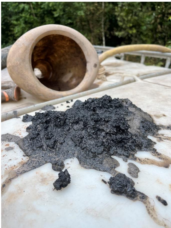
Station Works: 21/07/23 BH01A Coal Returns
