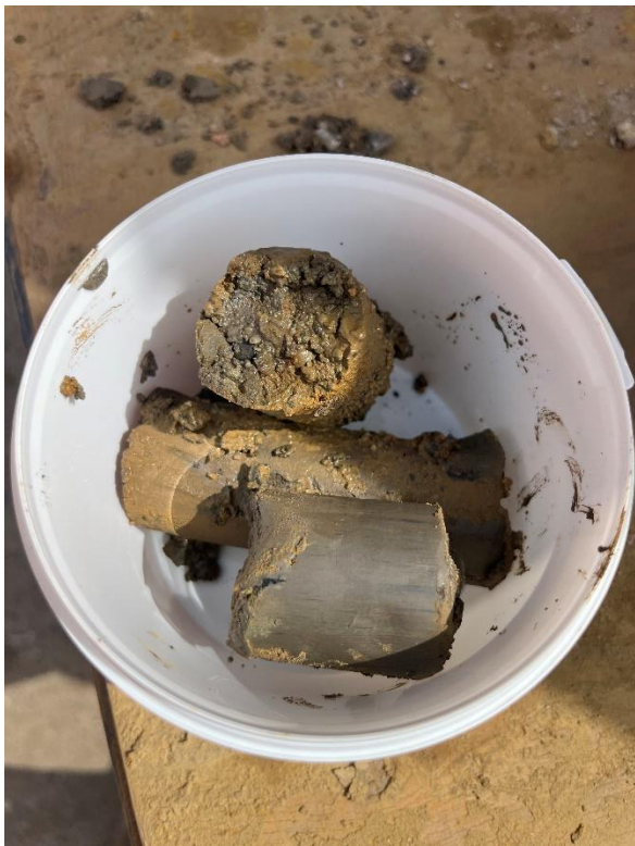
Station Works: 26/07/23 BH03 Stiff Clay 3.20m
