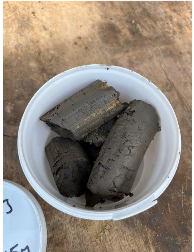
Station Works: 20/07/23 BH01 Stiff Clay 4.0m
