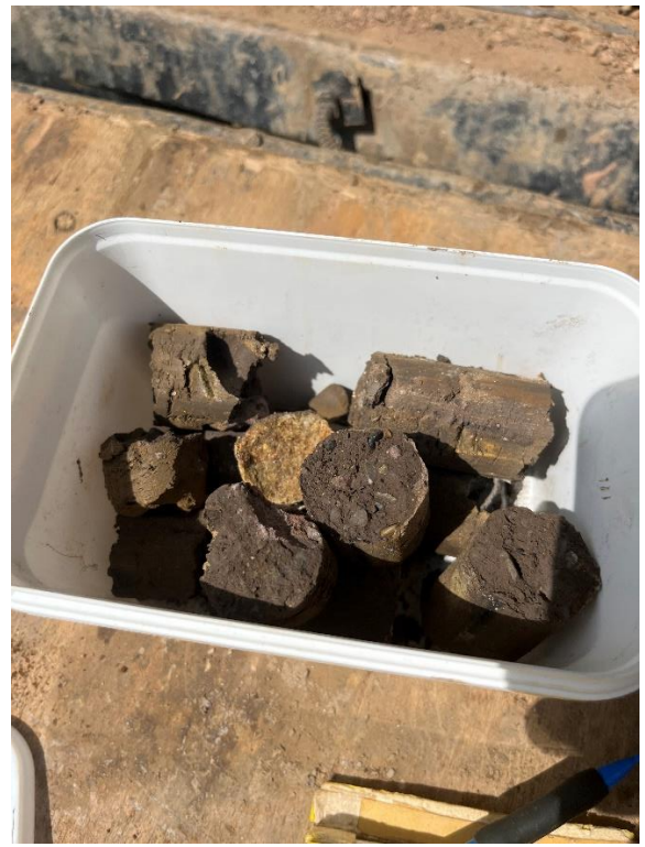
Station Works: 20/07/23 BH01A Hard Clay 10.50m
