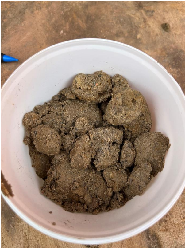
Station Works: 19/07/23 BH01 Natural Sand 1.20m
