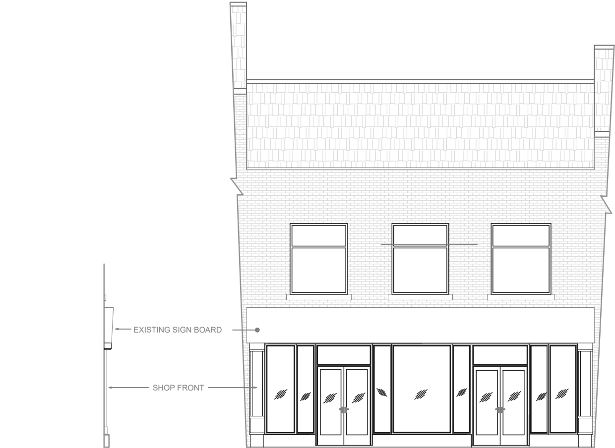
EXISTING SHOP FRONT & SIGNBOARD SIDE ELEVATION
