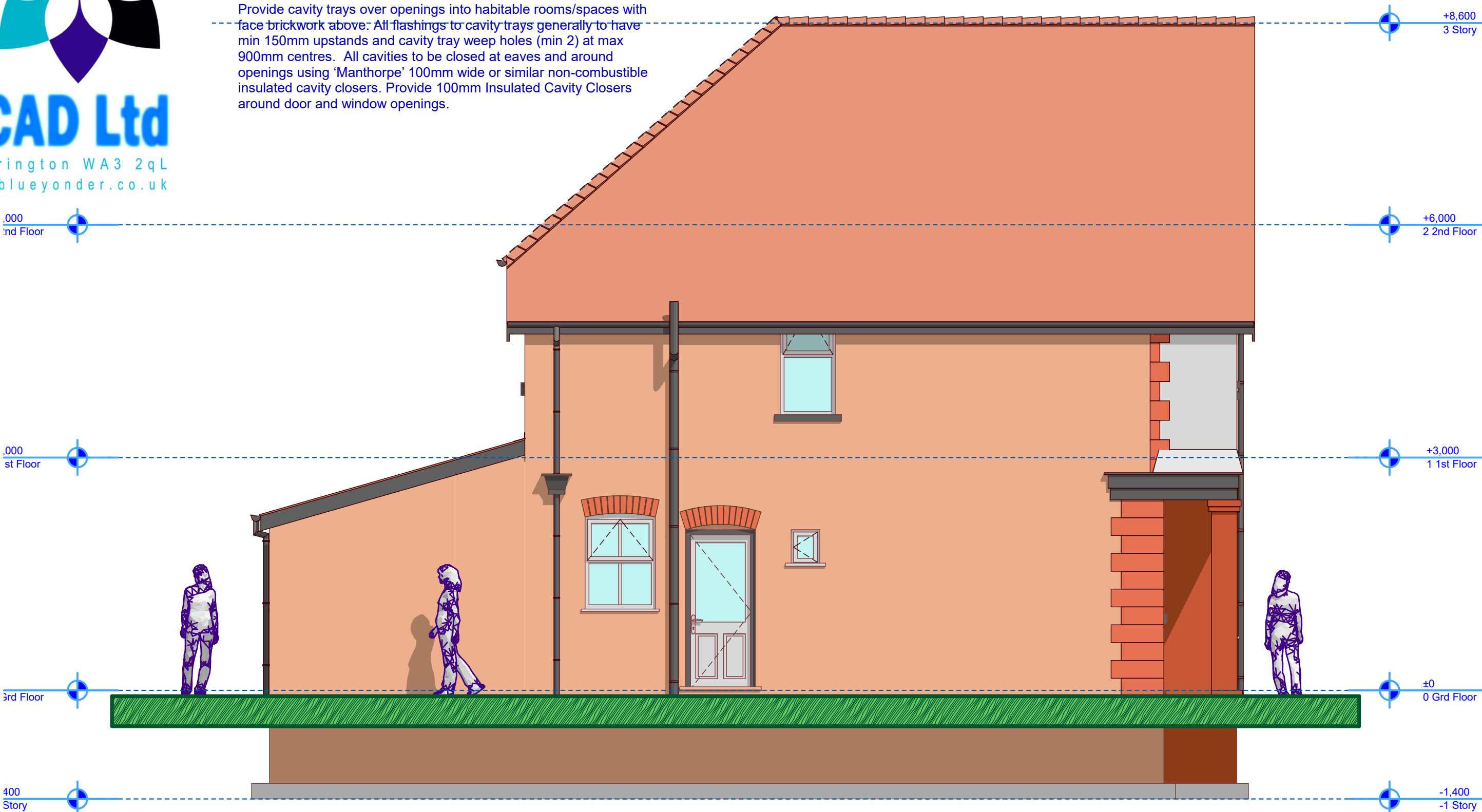
Existing Side Elevation
