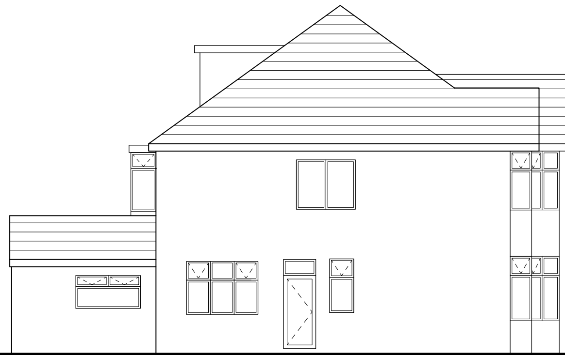
SOUTH ELEVATION SCALE 1:100 EXISTING - E009
